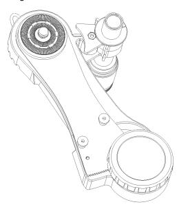
Point the mount to the Polaris. It is not important to be exactly aligned with the Polaris—a rough alignment is fine. Upon installing the supplied polar finder (B) we will look in more detail on how to have the star in the centre of the polar finder (B) field of view.
