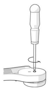
**7.2.** Release and unscrew the timer screw with washer (#10) using a Philips-style screwdriver (not included).
