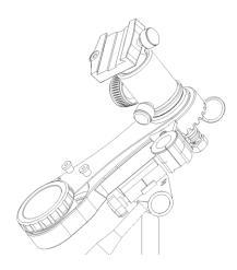
**4.4.** The ball-head must be securely fixed. Make sure to tighten it well. All the weight from the camera will rest on the ball-head. Besides that, a well-fixed ball-head ensures that there will be no slippage during long-exposures. At this point, it is important that the ball-head knobs are also tight. This prevents movement when installing the camera.
