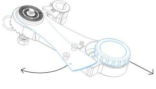
**7.3.** Push the winding knob (#6) away from the arm in order to slide the arm to the left – please push it slightly only and make sure the spring preventing this movement.
