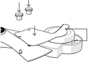
**7.6.** Place the South arm (C) and adjust it to the arm so the it is placed between the winding knob and the timer. Make also sure that the two protruding studs and the arm's thru holes are aligned. The Winding knob should move freely and be easily adjustable to the South arm's teeth.
