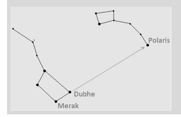
**5.3.** Peek through the polar finder (B) and centre Polaris in the visual field. Turn the tripod's fine-adjustment levelers to do so. Please read the following section for more details on how to correctly use the MiniTrack Quattro NS and the importance of correct balance.
