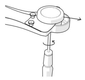
**7.8.** Push the arm to the timer and the winding knob against the teeth. Use a Philips-style screwdriver (not supplied) to fix it in place. It is important to not overtighten the screw as it may damage the timer and its performance.
