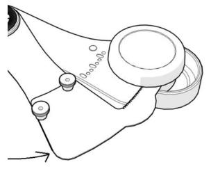
**7.7.** Push the assembled arm back to it's original position. Make sure to keep the winding knob remains "up-side down"
