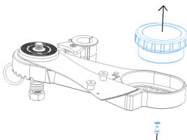
**7.4.** Remove the winding knob (#6) and the timer screw and washer (#10) as shown.
