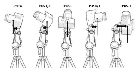
6.2. Pointing East. When the weight of the camera setup tends to rotate the ball-head in an anti-clockwise direction, the spring should be tensioned to one of the numbered teeth, based on how strong the imbalance is. By tensioning the spring in position 5 (worst case scenario) a weight of up to 4kg can be balanced – i.e. pointing to the Zenith with the camera body
