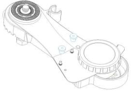
7.1. Release and remove the two thumbnuts (#8 Side A).
