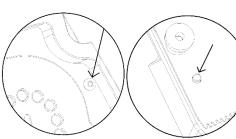
the Alignment through-hole (#8) as shown below. Now that it is locked you can thread the 3/8" threaded ball head (not included).
