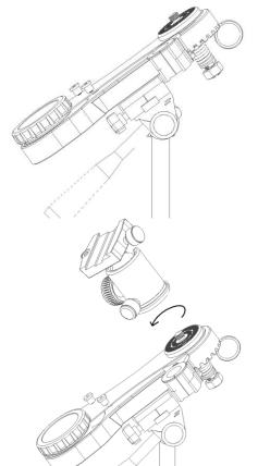
**4.2.** Make sure the mount is parallel to the adapter base. This is important because the inclination needs to be fine-tuned to set the mount in station. Check "how to set the mount into station" in 5.2. (for the Northern Hemisphere)
