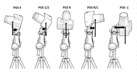
9.2. Pointing West. When the weight of the camera setup tends to rotate the ball-head in a clockwise direction, the spring should be tensioned to one of the castellations, based on how strong the imbalance is. By tensioning the spring in position +5 (worst case scenario) a weight of up to 4kg can be balanced – i.e. pointing to the Zenith with the camera body towards the west in respect to the ball-head.
