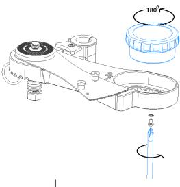
**7.5.** Turn the winding knob (#6) 180 degrees form it's original position (up-side down) and screw back the timer screw and washer (#12 Side B) but **do not tighten it yet!**
